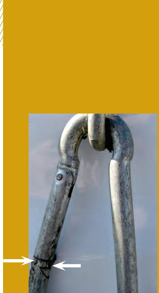
*While commonly used on chains, these connectors cannot stand the stress they will encounter during vehicle or equipment extraction. Notice how little metal there is on the post. This greatly weakens the connector.*
