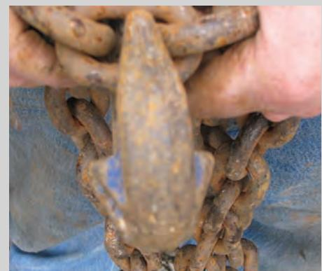
*Never use a chain if its hooks have been altered in any way or if the hooks' ratings are not equal to or greater than the chain's rating. Certain hooks have wings or ears on them to keep the chain from pinching too tight around the hook. It allows the force to be distributed on all links instead of just one.*
