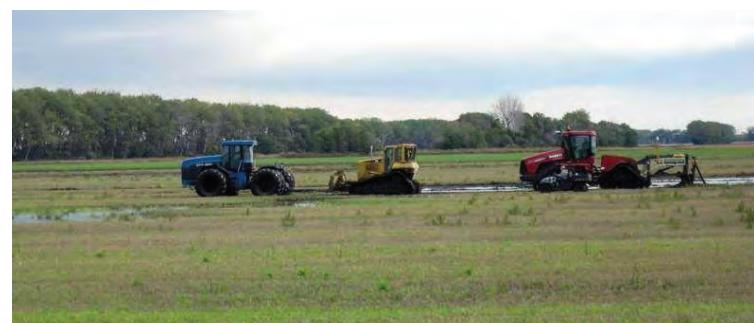
*There should never be another person in the danger zone when you are extracting a stuck vehicle. The person on the four-wheeler is in great danger because a piece of metal or strap could come lose during the pulling process.*
