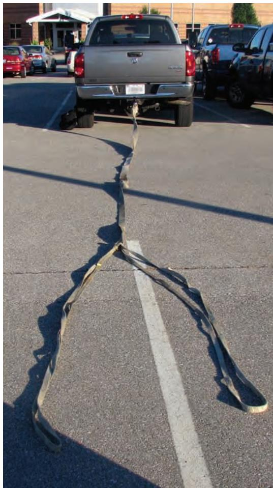
*Tying two or more recovery straps together with a knot reduces the overall towing power. The rope is at full strength when it is flat and the fiber is not pinched together. The strength of the strap is now based on the strength of the knot.*
