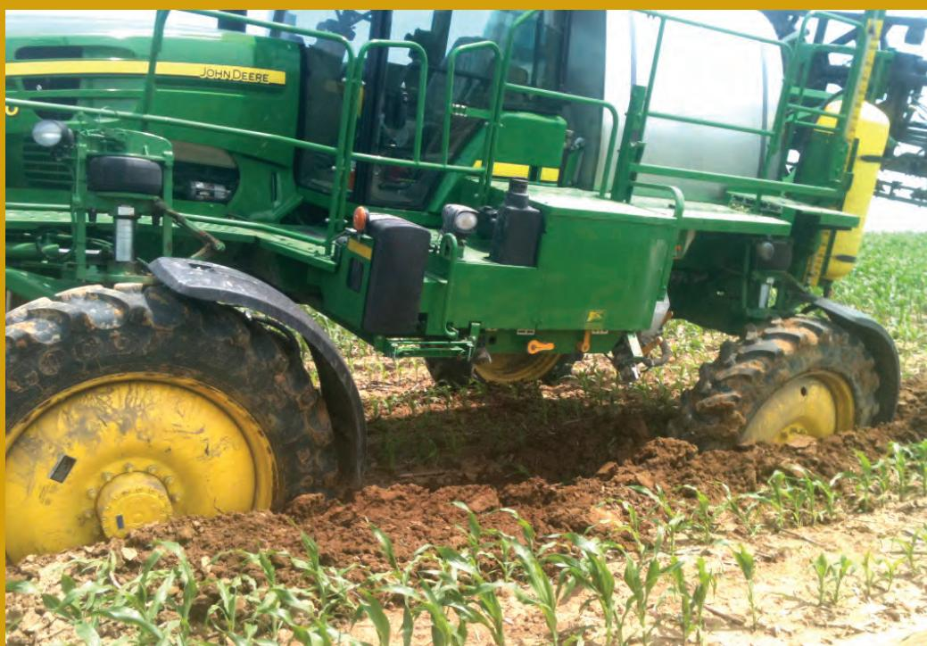
*Assume that this piece of equipment is being pulled out. It's important to determine whether the valve, speed sensor, or hose have been damaged.*
