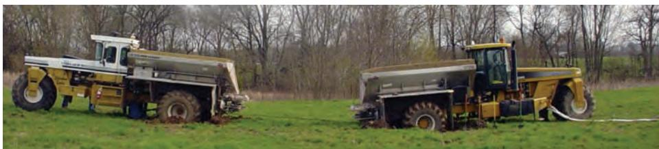
The two attachment points are to the towing vehicle and the stuck vehicle. It is not a good idea to hook multiple chains, straps, or ropes together. For instance, if you attached two, 30-foot ropes together, the real issue will be the clevis that connects the two ropes in the middle. The amount of force you generate could snap one of the ropes. If you need more length than what you have, call a wrecker service.
