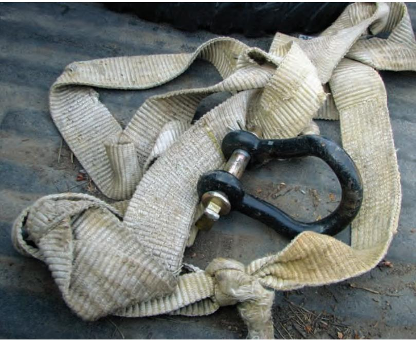
*This clevis is solid, but all its strength is defeated by knotting up the strap.*
