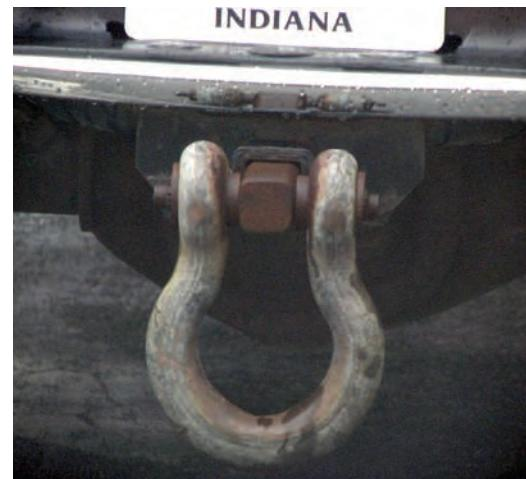
*This equipment looks impressive, but looks can be deceiving. Always look for the ratings associated with each piece of equipment. In this case, pay particular attention to the receiver hitch platform and make sure it is rated equal to or greater than the pickup.*
