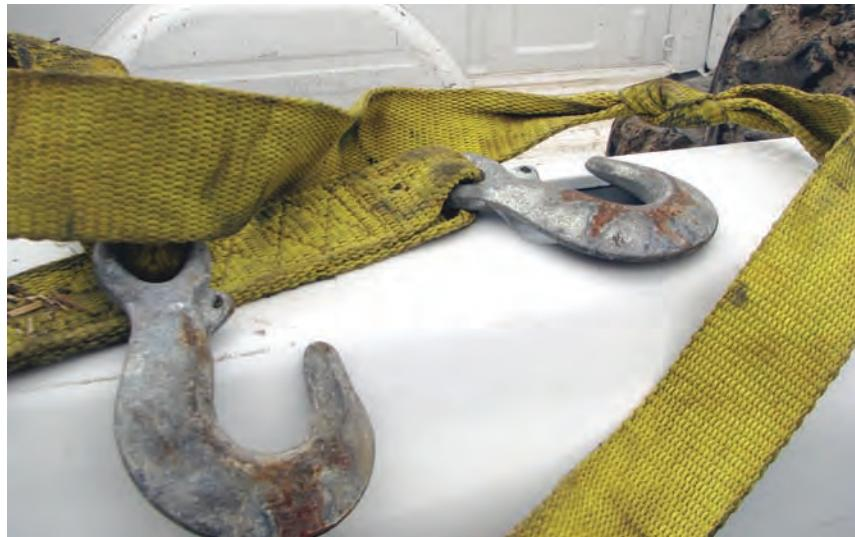
If you find serious defects, don't stick the equipment back in the truck or shop. If it's bad, make sure to discard or repair it so others will not be tempted to use it. Don't leave damaged equipment laying around to be used again — the next time it may be used, could be someone's last.
