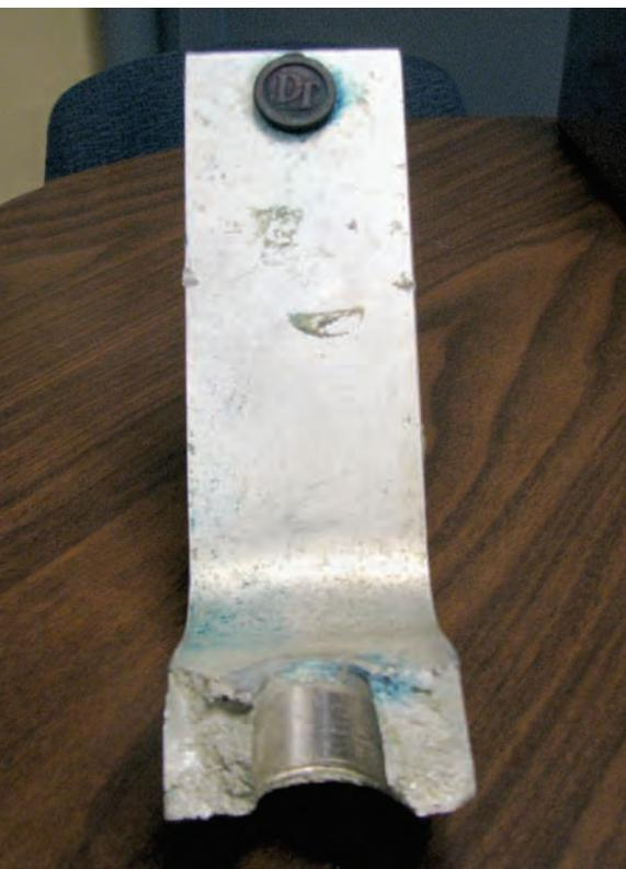
*An attempt was made to pull out a sprayer with the hitch. The force exceeded the ball, shank, and insert, which caused the metal to recoil into the equipment.*
