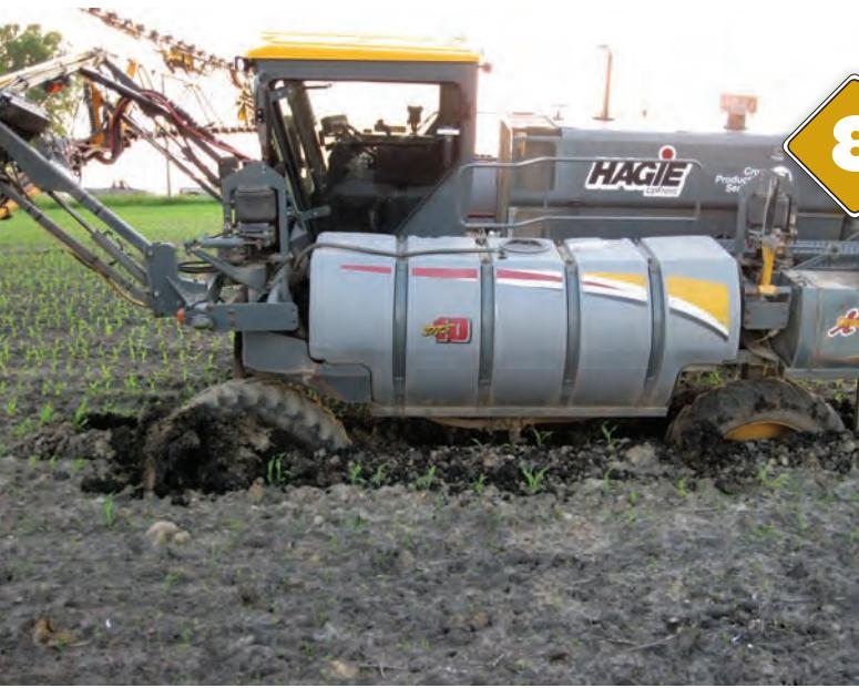
In some cases, it may be a good idea to lighten the load of the stuck vehicle. The lighter the vehicle you are pulling, the easier it will move and the less force it will have against your towing vehicle. Unloading stuck vehicles can also help prevent the stuck vehicle from getting top heavy if one side is down.
