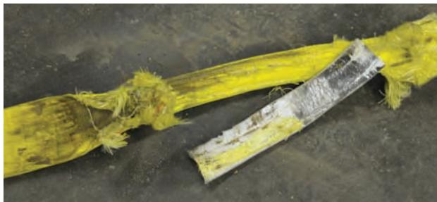
*Every device used to extract stuck equipment has a breaking point when it exceeds the rating of the device.*
