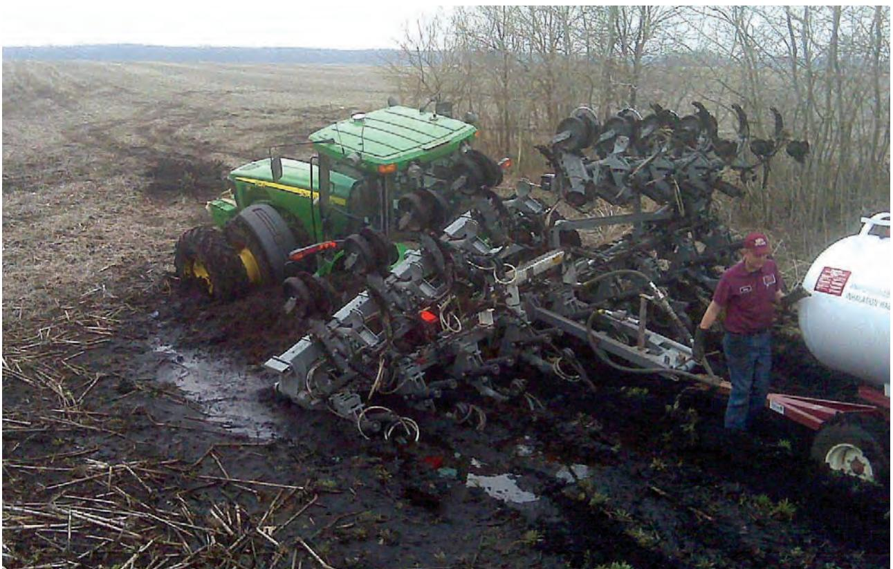
*You need to be especially careful in a situation like this. Inspect all hoses and fittings after the tractor and wagon are pulled out to make sure no anhydrous has leaked. And before you try to make any extraction consider whether the wagon should be separated from the tractor, the wagon should be pulled out backward, and the anhydrous ammonia tank valves have been shut off.*
