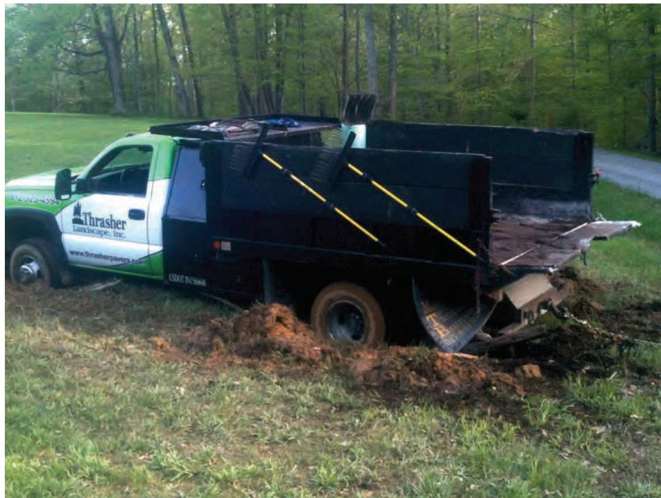
*When using a custom-made hitch, you need to know its strength. Putting boards and other objects under the tires can be dangerous if they are slung out.*
