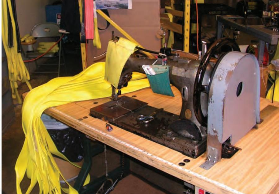
*Strap manufacturers can repair damaged straps. They can cut off the defective piece and sew on a replacement.*
