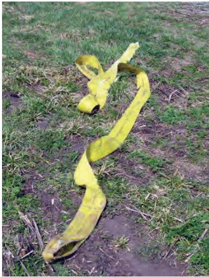
*Should the clevis be rated more than the rope or the strap? Many think that you want the rope to fail before the clevis. A rope failure is a lot better than a chain, cable, hook, or clevis flying through the air. You want the weakest link to be the rope or strap.*
