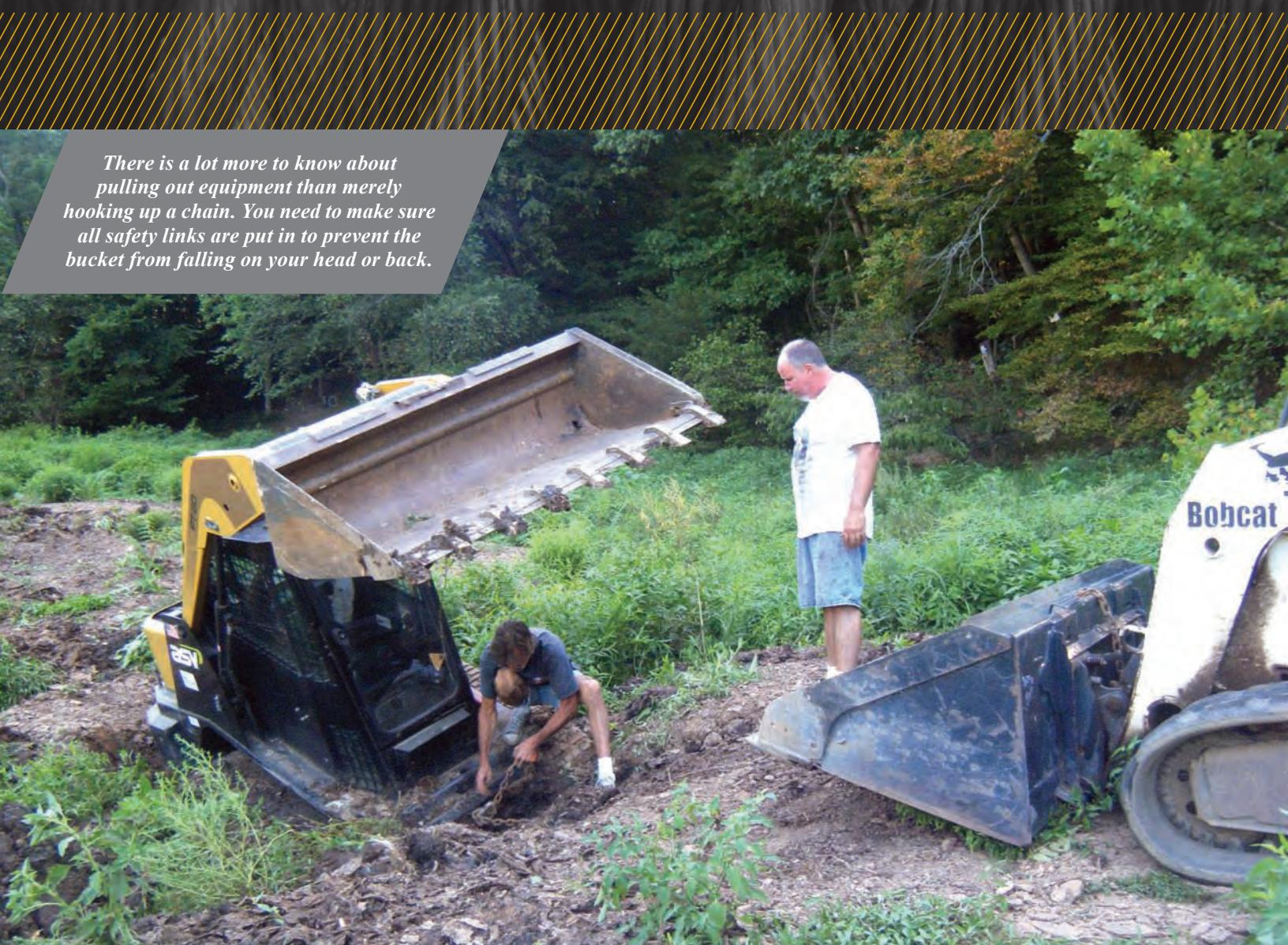
Before you try to extract any stuck vehicle with a cable, rope, or chain, consider the 28 tips described below. Remember, your goal is to have the pulling force exceed the immovable force — only then will the truck or stuck equipment move forward. If there is not enough force pulling forward, then whatever is stuck will not move.
