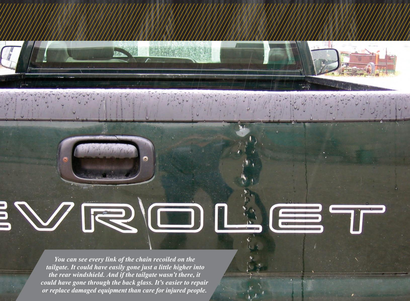
You can see every link of the chain recoiled on the tailgate. It could have easily gone just a little higher into the rear windshield. And if the tailgate wasn't there, it could have gone through the back glass. It's easier to repair or replace damaged equipment than care for injured people.
