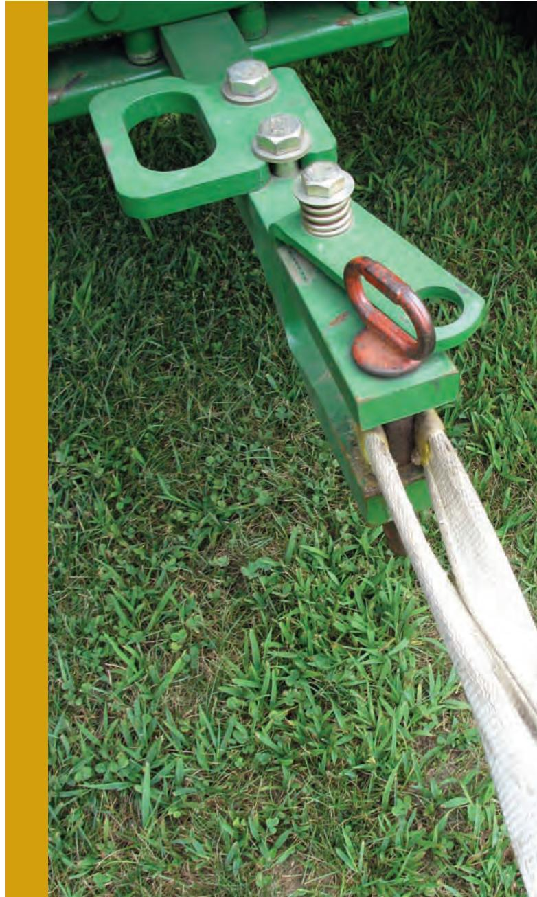
It is usually not a good idea to use a truck hitch to extract stuck equipment. In fact, many manufacturers' hitch tag instructions caution against using the hitch to pull out equipment.
