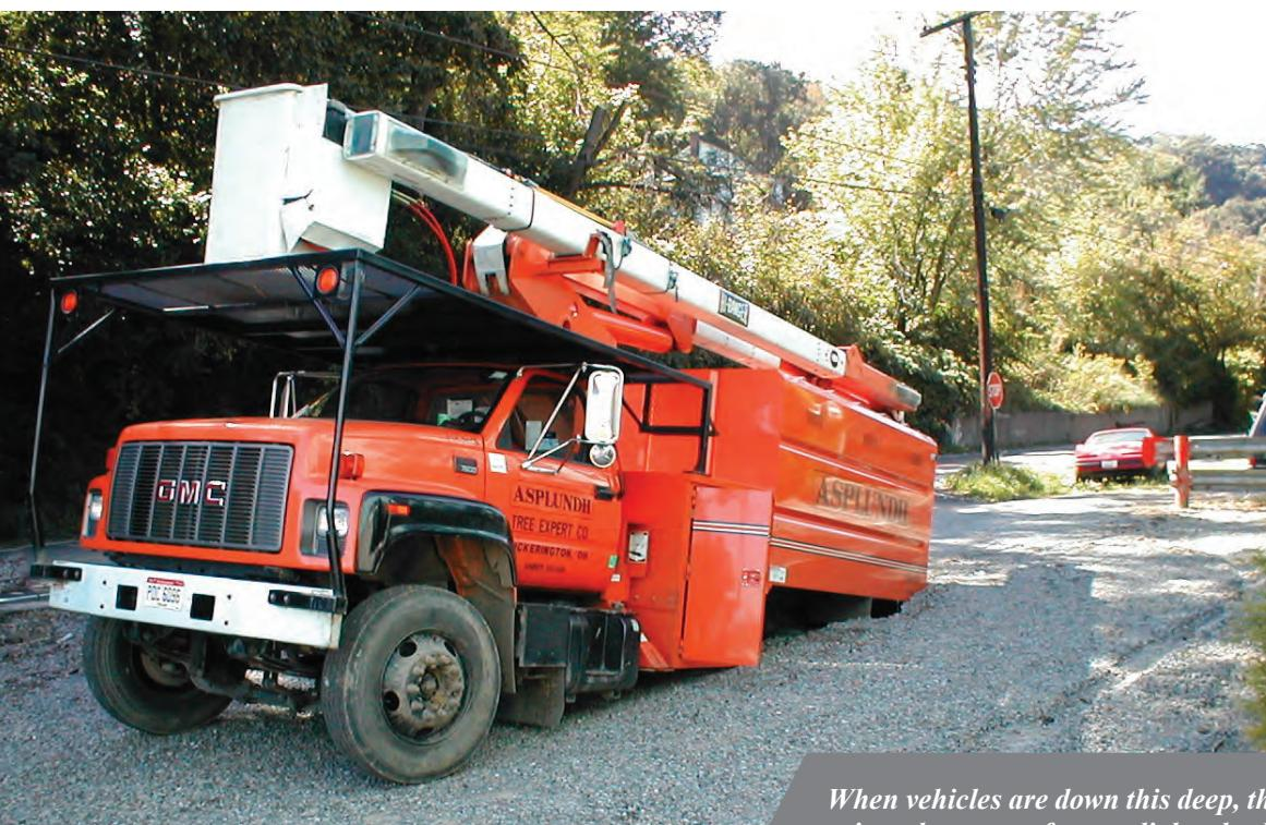
*When vehicles are down this deep, there could be serious damage to frames, lights, brake lines, tires, hitches, fuel tanks, and exhaust systems. Don't put defective equipment back on the road. Take a few minutes to inspect all equipment after any extraction.*
