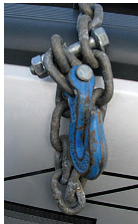
*Never make a loop at the end of a chain and attach it with a bolt. This compromises the strength of the chain. The chain's strength is no longer the weakest point or limiting factor. Now, all of the force will be placed on a loosely tightened nut. Bolts are made to work when they are tightened down for whatever they are holding. Use the chain and the hooks as they are intended to be used.*
