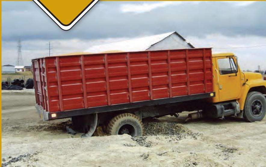
*Since this truck is loaded with corn, the total weight that needs to be pulled out will be a lot more than the truck alone.*
