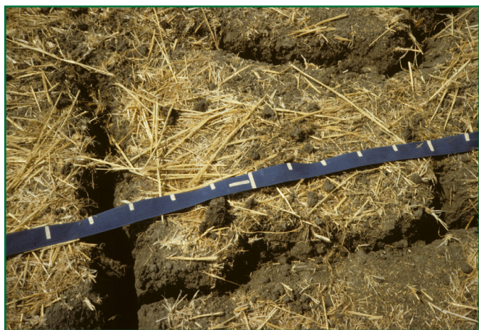
Figure 4. Surface cracks are good indicators of a soil that is prone to swelling and shrinking. Marks on the tape are approximately 4 inches apart.
